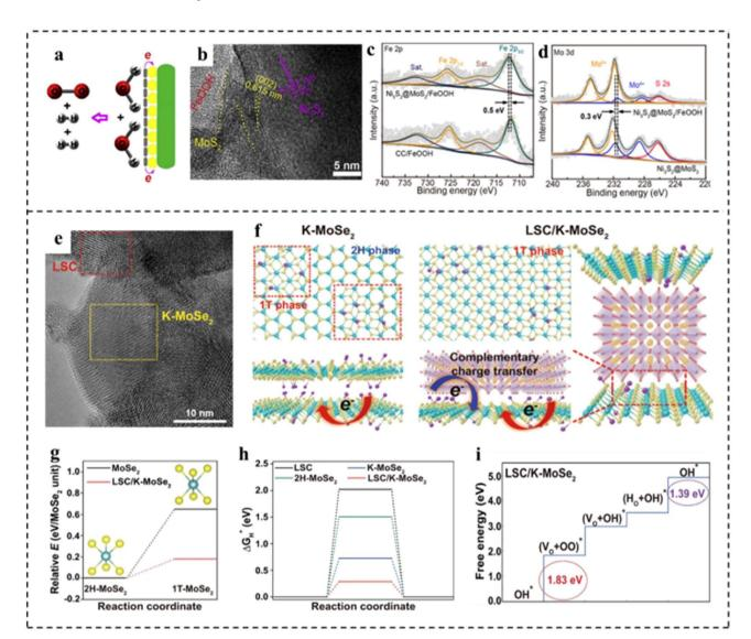
Fig. 17 (a) Schematic diagram for the overall water splitting mechanism of  $Ni_3S_2@MoS_2/FeOOH$ . (b) HRTEM image of  $Ni_3S_2@MoS_2/FeOOH$ . (c) Fe 2p XPS spectra of  $Ni_3S_2@MoS_2/FeOOH$  and FeOOH on carbon cloth (FeOOH/CC). (d) Mo 3d XPS spectra of  $Ni_3S_2@MoS_2/FeOOH$  and  $Ni_3S_2@MoS_2/FeOOH$  and  $Ni_3S_2@MoS_2/FeOOH$  and FeOOH on carbon cloth (FeOOH/CC). (d) Mo 3d XPS spectra of  $Ni_3S_2@MoS_2/FeOOH$  and  $Ni_3S_2@MoS_2/FeOOH$
