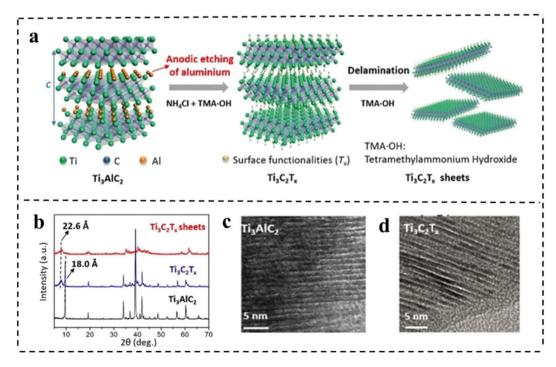
Fig. 11 (a) Schematic of the etching and delamination process of bulk  $Ti_3AlC_2$ . (b) XRD patterns of  $Ti_3AlC_2$  and  $Ti_3C_2T_x$ . HRTEM images of (c)  $Ti_3AlC_2$  and (d)  $Ti_3C_2T_x$ , respectively. Reproduced with permission from ref. 101. Copyright 2018, Wiley-VCH.
