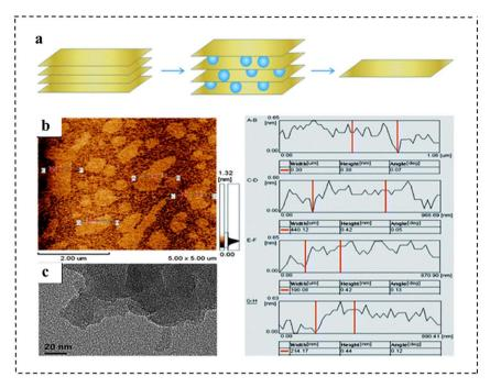
Fig. 7 (a) Illustration of the synthetic strategy of monolayer  $g-C_3N_4$  nanosheets. (b) AFM images and (c) TEM images of the as-prepared monolayer  $g-C_3N_4$  nanosheets. The right panel shows the height and width information of different nanosheets from the AFM images. Reproduced with permission from ref. 89. Copyright 2013, Royal Society of Chemistry.
