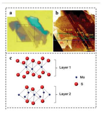
Fig. 10 (a) Optical micrograph of thin MoS<sub>2</sub> films deposited on the  $SiO_2/Si$  substrate. (b) AFM height image was taken for the 8  $\times$  8  $\mu m^2$ area indicated by dotted lines in (a). The thickness of each layer is shown by the height profile (in green) taken along the blue line in the AFM image. (c) Schematic model of the MoS<sub>2</sub> bilayer structure. Reproduced with permission from ref. 97. Copyright 2010, American Chemical Society.
