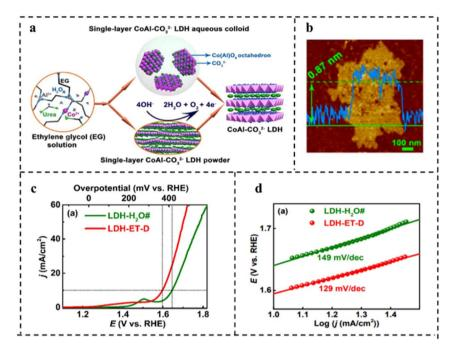
Fig. 14 (a) Schematic diagram of synthesis of water-dispersible single-layer  $CoAl-CO_3^2$  LDH. (b) AFM image of single-layer  $CoAl-CO_3^2$  LDH. (c) Polarization curves in  $O_2$ -saturated 1 M KOH at a scan rate of 0.5 mV s<sup>-1</sup>. (d) Tafel plots corresponding to (c). Reproduced with permission from ref. 116. Copyright 2017, American Chemical Society.
