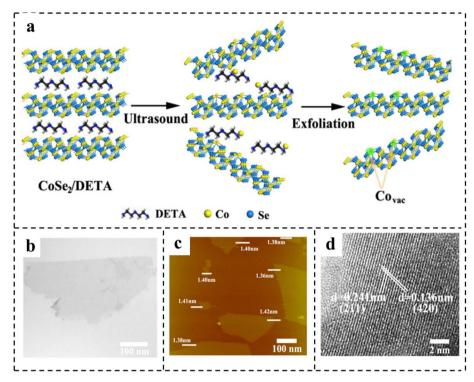
Fig. 6 (a) Schematic of the formation of vacancies in CoSe<sub>2</sub> ultrathin nanosheets. Characterization of CoSe<sub>2</sub> ultrathin nanosheets: (b) TEM image; (c) AFM image; (d) HRTEM image. Reproduced with permission from ref. 85. Copyright 2014, American Chemical Society.
