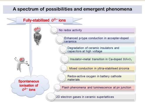
Fig. 10 Cartoon showing the range of possibilities and emergent phenomena between the zero conductivity of structures containing fully-stabilised  $O^{2-}$  ions and the free electrons in 2D electron gases at layer interfaces of artificial superlattices.
