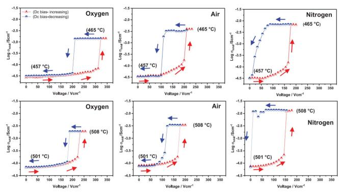
Fig. 9 Total conductivity at two temperatures and in atmospheres of different pO<sub>2</sub> of  $Hf_{0.85}Y_{0.15}O_{1.925}$  on a stepwise cycle of increasing and decreasing applied voltage after reaching a steady state at each voltage; reproduced from ref. 12: M. Alotaibi et al., J. Am. Ceram. Soc., 2023, 106, 822 with permission from Wiley publishing.
