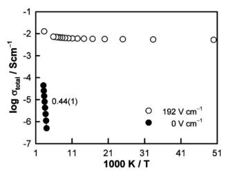
Fig. 8 Arrhenius plots of the total conductivity of Bi<sub>0.95</sub>Ca<sub>0.05</sub>FeO<sub>3</sub> measured without a *dc* bias and with an applied field of 192 V cm<sup>-1</sup>; reproduced from N. Maso et *al.*, *Phys. Chem. Chem. Phys.*, 2014, **16**, 19408 with permission from the PCCP owner societies.
