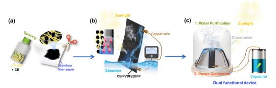
Fig. 1 Schematic illustrations of the interfacial evaporation system based on CB/PVDF@BFP for solar-driven water purification and evaporation-induced electricity generation. (a) Preparation process of the CB/PVDF@BFP material. (b) Working principles of the water purification and evaporation-induced power generation processes on the CB/PVDF@BFP platform upon sunlight irradiation. (c) Dual-functional device for concurrent solar-driven water purification and power generation.
