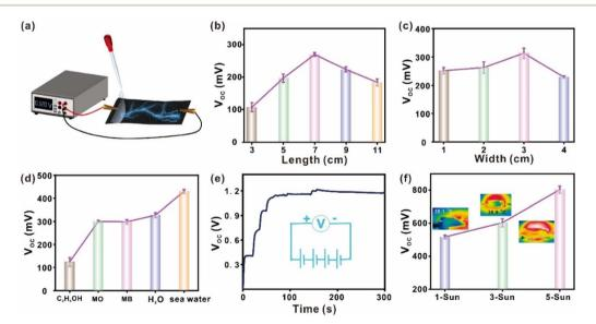
Fig. 3 Evaporation-induced electricity generation by the CB/PVDF@BFP platform. (a) Scheme depicting the experimental setup to characterize power generation performance.  $V_{\rm OC}$  of the CB/PVDF@BFP platform at various device (b) length, (c) width, and (d) when subjected to different liquids/solutions under 1 sun and 25 °C. (e)  $V_{\rm OC}$  of CB/PVDF@BFP platforms that are connected in series under 1 sun or (f) under different sunlight intensities (1–5 sun) at 25 °C. Insets: IR images.
