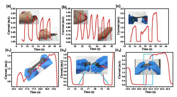
Fig. 5 Monitoring the changes of electrical signals during (a) finger and (b) elbow movements and (c-c<sub>3</sub>) material stretching under different tensile conditions based on the APC-PVA@ZnCl2 sensor.
