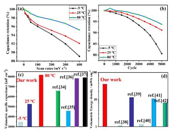
Fig. 4 (a) Capacitance retention of APC-PVA@ZnCl2 (a) at different temperatures and scan rates. (b) After experiencing 5000 cycles. (c and d) Comparison maps of volumetric specific capacitance and energy density of APC-PVA@ZnCl2 with reported work.
