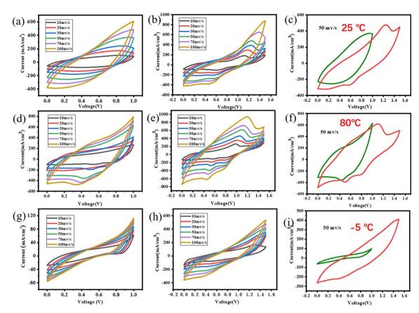
Fig. 3 (a, d and g) Typical CV curves of APC-PVA@ZnCl<sub>2</sub> at different temperatures between the potential range of 0 and 1 V and at different scanning rates, (b, e and h) Typical CV curves of APC-PVA@ZnCl<sub>2</sub> with different scanning rates between the potential range of 0 and 1.6 V at different temperatures, (c, f and i) CV contrast diagram under various potential windows at different temperatures at a scan rate of 50 mV s<sup>-1</sup>
