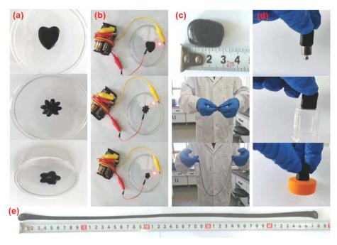
Fig. 6 (a) Digital photograph of the plasticity of APC-PVA@ZnCl<sub>2</sub> materials; (b) electrical conductivity; (c) stretchability; (d) adhesion; (e) tensile length.
