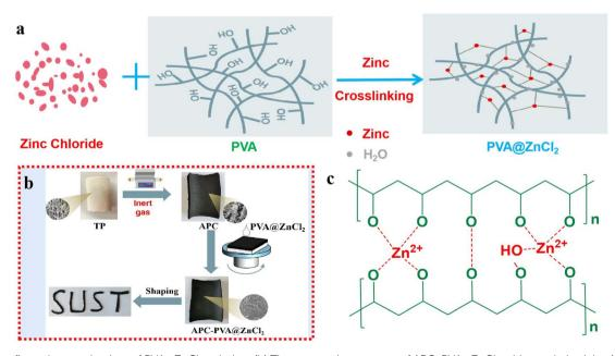
Fig. 1 (a) Configuration mechanism of PVA@ZnCl<sub>2</sub> solution. (b) The preparation process of APC-PVA@ZnCl<sub>2</sub> with good plasticity. (c) The crosslinking mechanism between PVA and  $Zn^{2+}$ .
