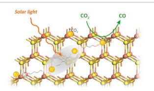
Fig. 5 Schematic illustration of CdS nanorods with S vacancies for photocatalytic  $\rm CO_2$  to CO conversion.
