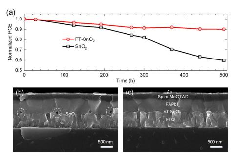
Fig. 5 (a) Comparison of normalized PCE of PSCs based on bare  $SnO_2$  and  $FT-SnO_2$ . The devices were stored in the dark at room temperature and under relative humidity of  $25 \pm 10\%$  for 500 h. Cross-sectional SEM images of the 500 h-aged PSCs based on (b) bare  $SnO_2$  and (c)  $FT-SnO_2$ .
