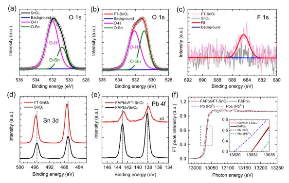
Fig. 1 O 1s XPS data for (a) bare  $SnO_2$  and (b)  $SnO_2$  modified with 4-fluorothiophenol (FT- $SnO_2$ ). (c) F 1s and (d) Sn 3d XPS spectra of bare  $SnO_2$  and FT- $SnO_2$ . (e) Pb 4f XPS spectra and (f) Pb  $L_3$  edge XANES spectra of FAPbl $_3$  black powder and FAPbl $_3$ -coated FT- $SnO_2$  powder. XANES spectra of metal Pb and Pbl $_2$  were measured for reference. Inset shows XANES data of the rectangular dashed line region.
