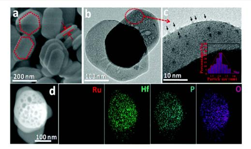
Fig. 25 Solid state imaging ((a): SEM; (b and c): TEM; (d): HAADF-STEM) and elemental mapping of active Ru/α-HfP catalyst. Reproduced from ref. 38 with permission from RSC, copyright 2019.
