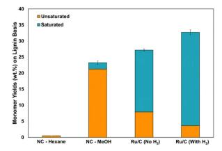
Fig. 22 Effects of pressurized hydrogen on monomer yields in reductive catalytic fractionation of herbaceous biomass. Reproduced from ref. 109 with permission from ACS, copyright 2018.
