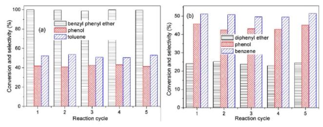
Fig. 19 (a) Reusability tests for hydrogenolysis of benzyl phenyl ether using Au<sub>1</sub>Pd<sub>1</sub>/CeO<sub>2</sub>. (b) Reusability tests for hydrogenolysis of diphenyl ether with Au<sub>1</sub>Pd<sub>1</sub>/CeO<sub>2</sub>. Reproduced from ref. 81 with permission from Elsevier, copyright 2021.
