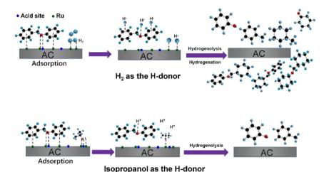
Fig. 12 Proposed pathway for catalytic hydrogenolysis of BPE over Ru/AC. Reproduced from ref. 75 with permission from Elsevier, copyright 2021.
