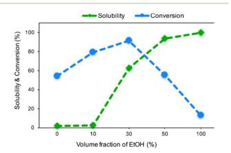
Fig. 7 Solubility of BPE and its conversion in different volume fractions of  $H_2O/EtOH$  co-solvent system. Reproduced from ref. 53 with permission from RSC, copyright 2019.
