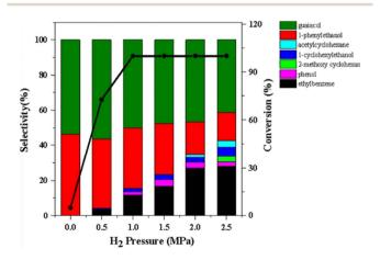
Fig. 4 The product distributions for the conversion of 2-(2-methox-yphenoxy)-1-phenylethanol ( $\beta$ -O-4) over Ni/CaO-H-ZSM-5(60) under different H $_2$  pressures. Reproduced from ref. 52 with permission from BMC *Chem.*, copyright 2019.
