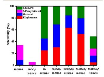
Fig. 8  $\beta$ -O-4 catalytic hydrogenolysis product distribution histogram. Reproduced from ref. 44 with permission from Elsevier, copyright 2020.
