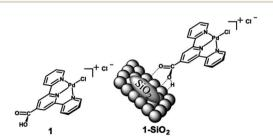
Fig. 16 Structure of chloro(2,2':6',2"-terpyridine-4'carboxylic acid) palladium(II) chloride (1) and a graphical representation of the molecular catalyst attached to a SiO<sub>2</sub> support (1-SiO<sub>2</sub>). Figure taken from reference. Reproduced from ref. 17 with permission from ACS, copyright 2019
