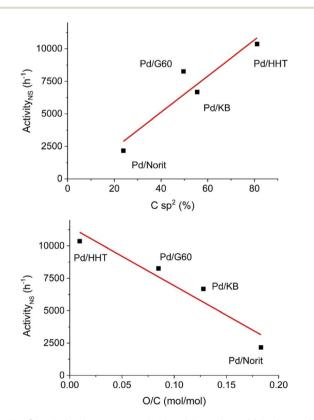
Fig. 13 Correlation between catalytic activity and graphitization order (top) and correlation between catalytic activity and oxygen functionalization (bottom). Reproduced from ref. 78 with permission from ACS, copyright 2019
