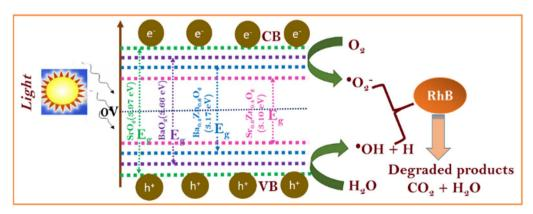
Scheme 1 Photocatalytic mechanism of BaO<sub>2</sub>, Ba<sub>0.4</sub>Zn<sub>0.6</sub>O<sub>2</sub>, SrO<sub>2</sub>, and Sr<sub>0.6</sub>Zn<sub>0.4</sub>O<sub>2</sub>.
