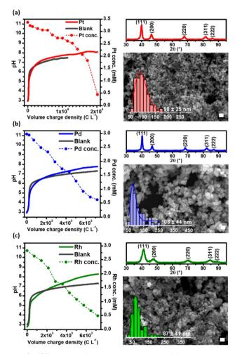
Fig. 1 (Left) Evolution of pH and concentration of dissolved platinum group metal ions as a function of the charge consumed per unit volume of catholyte, throughout the GDEx process yielding elemental nanoparticles. (Right) X-ray diffraction patterns (up) and SEM micrographs and distribution histograms (down) of the elemental nanoparticles. The white scale bar is 250 nm. (a) Pt; (b) Pd; (c) Rh.
