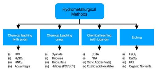
Fig. 6 Hydrometallurgical processes.
