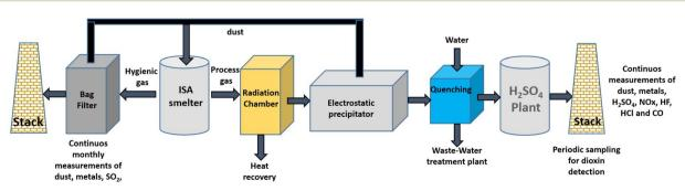
Emission control of the Isa Smelt furnace (adapted from Cui and Zhang, 2008)
