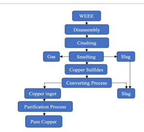
Fig. 4 Schematic flow chart of the smelting process.
