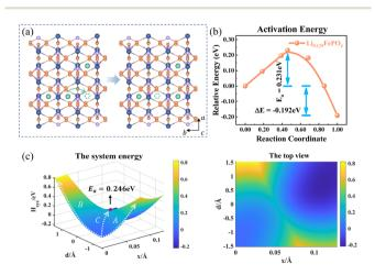
Fig. 5 (a) Structure diagram of the initial and final states of  ${\rm Li}^+$  hopping. (b) The activation energy calculated using the NEB for asymmetric ion hopping in  ${\rm Li}_{0.125}{\rm FePO}_4$ , and (c) potential energy surface based on the Hamiltonian model (left) and its top view (right) for ion transport and electron transfer.
