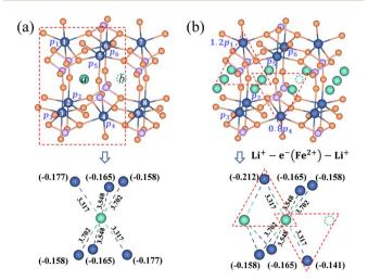
Fig. 3 Partial charges of an electron for (a) the isolated state and (b) the aggregated state of  $Li^+$  in the LiFePO<sub>4</sub> structure. The dimension unit of  $Li^+-e^-$  (Fe<sup>2+</sup>) distance is Å.
