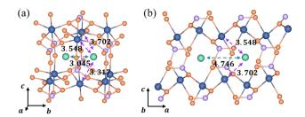
Fig. 6 Structural diagrams of  ${\rm Li}^+$  aggregation (a) in the [010] direction and (b) in the [100] direction; purple and green arrows represent electrostatic attraction and repulsion, respectively. The dimension unit is Å
