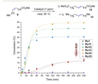
Scheme 3 Self-metathesis of methyl oleate (9, 95% pure). Conversion =  $100 \times [1 - (A_9 \times A_{\rm IS}^0)/(A_9^0 \times A_{\rm IS})]; A_9^0, A_{\rm IS}^0 = GC$  area of methyl oleate and internal standard before the reaction. Lines are visual aids only.
