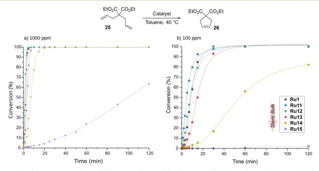
Scheme 6 Time/conversion curves for the RCM reaction of diethyl 2,2-diallylmalonate (25, 99% pure) with 1000 ppm of CAAC-based complexes (monitored by GC). Lines are visual aids only.
