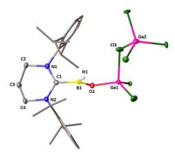
Fig. 2 The molecular structure of  $2 \cdot \text{GaCl}_3$ . Hydrogen atoms (except the hydrogen attached with boron atom) are omitted for clarity. Selected bond distances (Å), bond angles (deg), and torsion angle (deg): C1-N1 1.328(3), C1-N2 1.328(3), B1-C1 1.621(4), B1-O1 1.307(3), B1-H1 1.09(3), Ga1-O1 1.807(2), Ga1-Cl3 2.3015(10); N1-C1-N2 122.1(2), N1-C1-B1 118.5(2), C1-B1-O1 118.3(2), C1-B1-H1 117.6(17), B1-O1-Ga1 127.97(18), Ga1-Cl3-Ga2 117.49(4).
