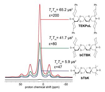
Fig. 4 Proton enhancement and saturation factors measured for 16 mM bTbK, bCTbK and TEKPOL in frozen solution of TCE at 100 K. The black spectrum is the microwave off signal. Adapted from ref. 70.
