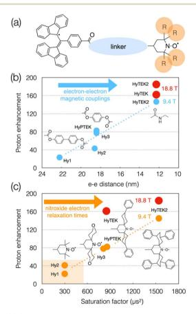
Fig. 8 (a) Schematic structure of BDPA-nitroxide hybrid radicals. (b) and (c) Plots showing the evolution of the enhancement factor with electron–electron distance (b) and saturation factor (c) in the HyTEK series. The blue and orange dots correspond to data acquired at 9.4 T, while the red dots are values measured at 18.8 T. Adapted from ref. 113.
