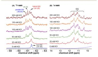
Fig. 8 (A)  $^{19}$ F NMR and (B)  $^{1}$ H NMR spectra of mutated modified ON 5 at different KCl concentrations. Peak at -61.03 could not be assigned.
