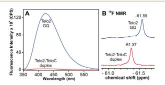
Fig. 3 (A) Fluorescence and (B)  $^{19}$ F NMR spectra of telomeric GQ and duplex structures. See the ESI† for experimental conditions.
