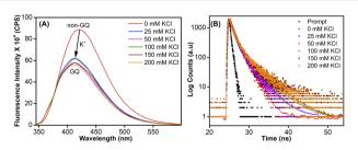
Fig. 7 (A) Steady-state and (B) time-resolved fluorescence spectra of modified ON 5 at different KCl concentrations. For steady state fluorescence, samples (1  $\mu$ M) were excited at 330 nm with excitation and emission slit widths of 5 nm and 6 nm, respectively. The instrument response (prompt) is shown in grey dots and decay curve fits are shown in solid lines.
