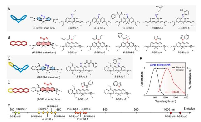
Fig. 2 Regulation  $\pi$ -electron delocalization induced spectral shift in Si-rhodamine fluorophores. Chemical structures of (A and C) bent-Si-rhodamine (B-SiRhd) and (B and D) planar-Si-rhodamine (P-SiRhd) fluorophores. (E) Normalized absorption and fluorescence spectra of representative asymmetric P-SiRhd-7 with a large Stokes shift. (F) Emission maxima peaks of bent/planar Si-rhodamines are visualized graphically on the electromagnetic spectrum.
