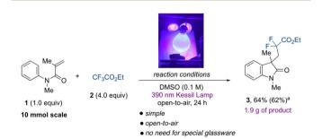
Fig. 4 Scalability of the defluorinative alkylation protocol for the large-scale preparation of difluorinated oxindoles.  $^{a}$ Yield for the 0.1 mmol scale reaction using 4.0 equiv. of 2. ArSH = 4-methoxybenzenethiol.
