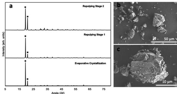
**Fig. 2** (a) XRD diffractogram of nickel sulfate crystals obtained after evaporative crystallization, repulping stage 1, and repulping stage 2. (b) and (c) SEM images of crystals obtained after evaporative crystallization. Scale bar: (b) 50  $\mu\text{m}$  and (c) 10  $\mu\text{m}$ .
