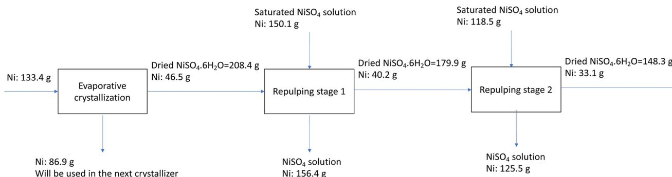
Fig. 4 Block flow diagram of the process and Ni mass balance.
