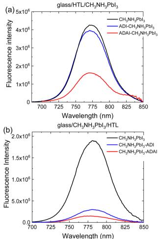
Fig. 7 Photoluminescence spectra registered by excitation of the perovskite through the HTL interface. The relative position of the HTL with respect to the perovskite is indicated
