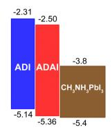
Fig. 3 Energy levels at the HTL/perovskite interface.
