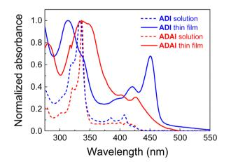
Fig. 2 Normalized absorption spectra in DMF solution ( $2.5 \times 10^{-5}$  M) and as thin films on quartz substrates, deposited by thermal evaporation in high vacuum  $(10^{-7}-10^{-8} \text{ mbar})$ .
