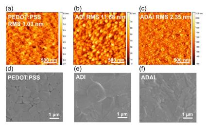
Fig. 6 (a-c) Tapping mode  $2 \mu m \times 2 \mu m$  atomic force microscopy images of the indicated HTL on ITO; (d-f) Top-view scanning electron microscopy images of the perovskite layer coated on the indicated HTL.
