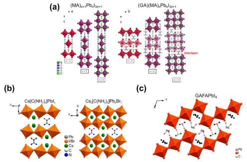
Fig. 6 Crystal structures of (a)  $(MA)_{n+1}Pb_nI_{3n+1}$  and  $(GA)(MA)_nPb_nI_{3n+1}$  (right), n=1, 2 and 3. Reproduced with permission. <sup>56</sup> Copyright 2017, ACS Publishing Group. (b)  $(GA)(Cs)_n Pb_n X_{3n+1}$  (n=1 and 2; X=I and Br) Reproduced with permission. <sup>57</sup> Copyright 2017, ACS Publishing Group; (c) GAFAPbl<sub>4</sub>. Reproduced with permission.<sup>34</sup> Copyright 2018, ACS Publishing Group.
