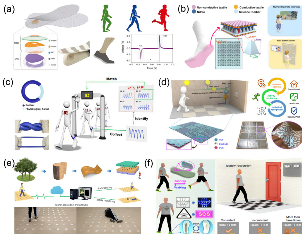
Fig. 6 TENG-based self-powered intelligent sensors for monitoring gait characteristics. (a) TENG-based wearable smart insole for real-time multifunctional gait monitoring. Reprinted with permission from ref. 37. Copyright 2019, Wiley-VCH. (b) Deep learning-enabled triboelectric smart socks for gait analysis. Reprinted with permission from ref. 98. Copyright 2020, Springer Nature. (c) Soft and stretchable triboelectric band for self-powered gait pattern-based identity recognition. Reprinted with permission from ref. 100. Copyright 2018, Elsevier B.V. (d) Deep learning-enabled smart mats as a scalable floor monitoring system. Reprinted with permission from ref. 38. Copyright 2020, Nature Publishing Group. (e) Self-powered smart floor system with path analysis and safety monitoring functions. Reprinted with permission from ref. 101. Copyright 2022, American Chemical Society. (f) TENG-based self-powered electronic textiles for an intelligent footwear system and identity recognition carpet. Reprinted with permission from ref. 102. Copyright 2020, Nature Publishing Group.
