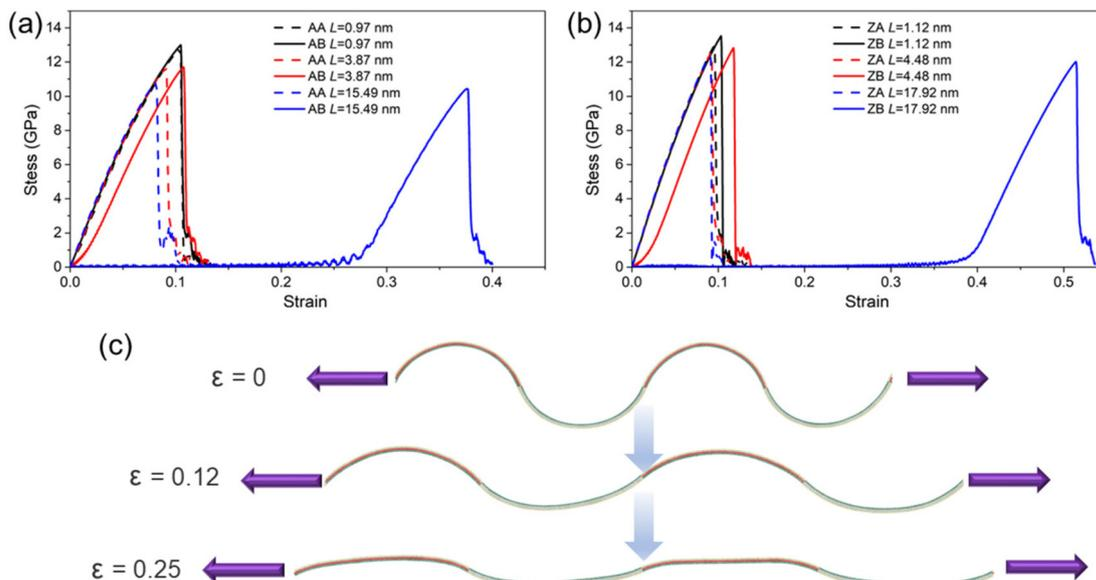
Fig. 5 The calculated stress–strain curves of the MoSSe/WSe heterostructure superlattice with (a) armchair and (b) zigzag interfaces with different lengths  $L$ ; (c) the side view of the structural evolution schematic for the AB MoSSe/WSe heterostructure under uniaxial tension.
