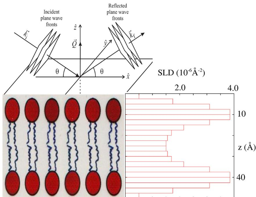
**Fig. 3** Schematic showing incident and reflected neutron waves in the specular condition. The picture is meant to represent a lipid bilayer with head (red ellipsoids) and tails for which a model SLD profile is plotted to the right.
