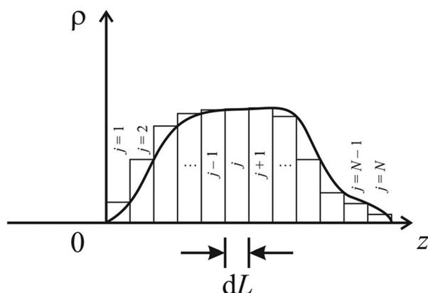
**Fig. 2** The solution method for a single slab, as described in the main body of text, can be extended to a SLD profile of arbitrary shape that is rendered into a series of consecutive slabs, each of thickness  $dL$  and characterized by its own particular value of SLD. (After Fig. 1.6 of Majkrzak et al.<sup>11</sup>).
