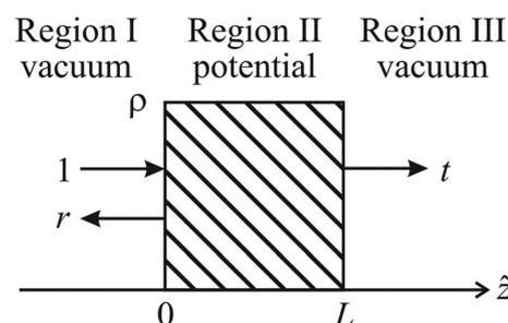
**Fig. 1** Schematic for specular reflection showing the incident or fronting region on the left, the scattering potential within the middle region, and the backing region on the right. The incident wave amplitude is taken to be unity whereas the reflected and transmitted amplitudes are designated to be  $r$  and  $t$ , respectively. (After Fig. 1.4 of Majkrzak *et al.*<sup>11</sup>).
