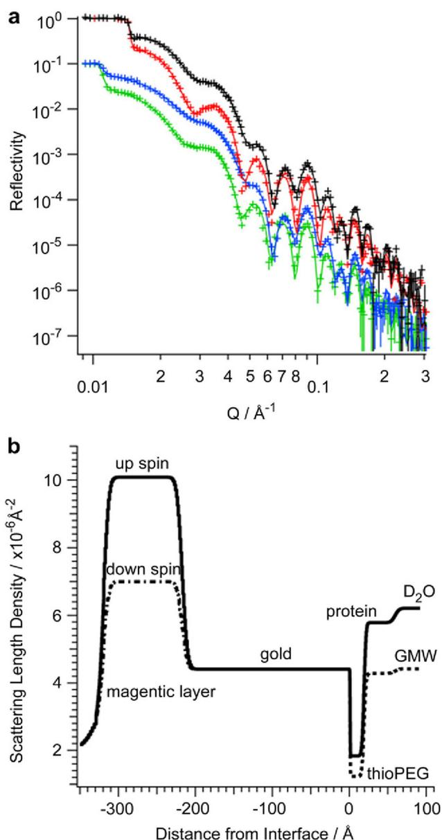
**Fig. 12** (a) The reflectivity of an array of ctOmpA in  $D_2O$  (black for neutron spin up and red for spin down) and gold SLD-matched water (GMW) (blue for neutron spin up and green for spin down). The symbols represent the data and the solid lines the fits. The GMW data is offset for clarity. (b) The corresponding SLD profile of the ctOmpA array. (After Fig. 4 of Le Brun *et al.*<sup>28</sup>).
