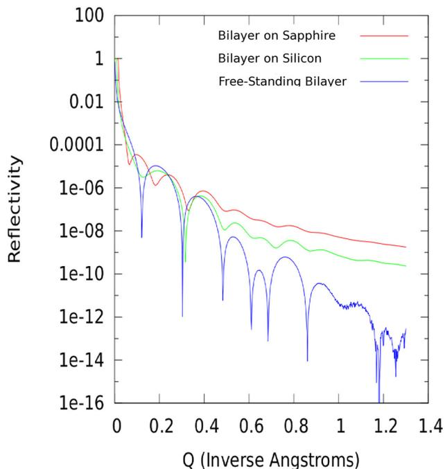
**Fig. 4** Calculated neutron reflectivity patterns corresponding to the lipid bilayer model SLD profile plotted in Fig. 3 as supported by sapphire ( $\text{Al}_2\text{O}_3$ ), silicon, or free-standing. The higher the value of the wavevector transfer  $Q$  at which reflectivity can be measured, the finer the spatial resolution that can be obtained in the corresponding depth profile.
