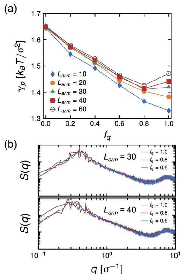
Fig. 11 Interfacial tension,  $\gamma_p$ , as a function of degree-of-protonation,  $f_q$ , for  $N_{\text{arm}} = 4$ ,  $\phi_s = 0.096$  and at different arm degrees-of-polymerization,  $L_{\text{arm}}$  (a). Scattering of the in-plane structure of PS beads,  $S(q)$  for  $L_{\text{arm}} = 30$  and 40 at  $f_q$ 's of 0.6, 0.8 and 0.1 (b).
