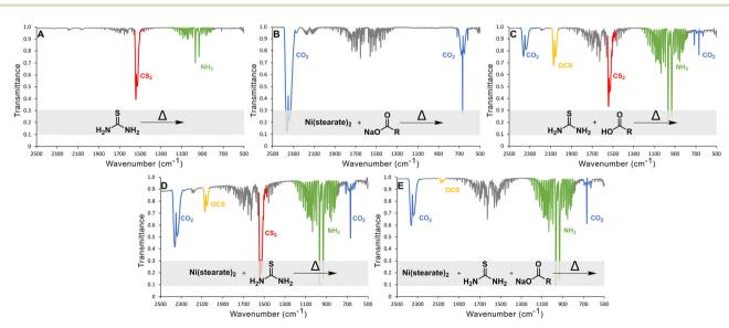
Fig. 3 Gas FTIR of thermal decomposition products of (A) thiourea (13.1 mmol) in ODE at 206 °C, (B) nickel stearate (0.5 mmol) and sodium oleate (3 mmol) in ODE at 210 °C, (C) thiourea (13 mmol) and oleic acid (13 mmol) in ODE at 213 °C, (D) nickel stearate (0.5 mmol) and thiourea (3 mmol) in ODE at 212 °C, and (E) nickel stearate (0.5 mmol), thiourea (3 mmol), and sodium oleate (3 mmol) in ODE at 200 °C.
