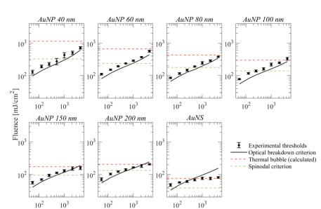
Fig. 6 Results of numerical simulations obtained by eqn (S2) (ESI†) and comparison to experimental measurements (black circles).
