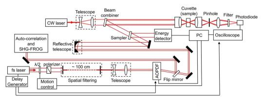
Fig. 1 Graphical representation of the experimental setup (see text for details).
