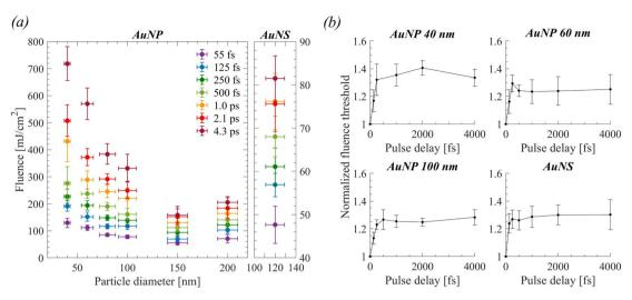
Fig. 3 (a) Size-dependent, experimentally evaluated fluence thresholds of detectable cavitation bubbles of spherical AuNPs (left) and the ones of AuNS (right) for all applied laser pulse widths. (b) Results of double 55 fs pulse experiments as a function of pulse delay. All fluence thresholds have been normalized to the one acquired under single 55 fs pulse excitation.
