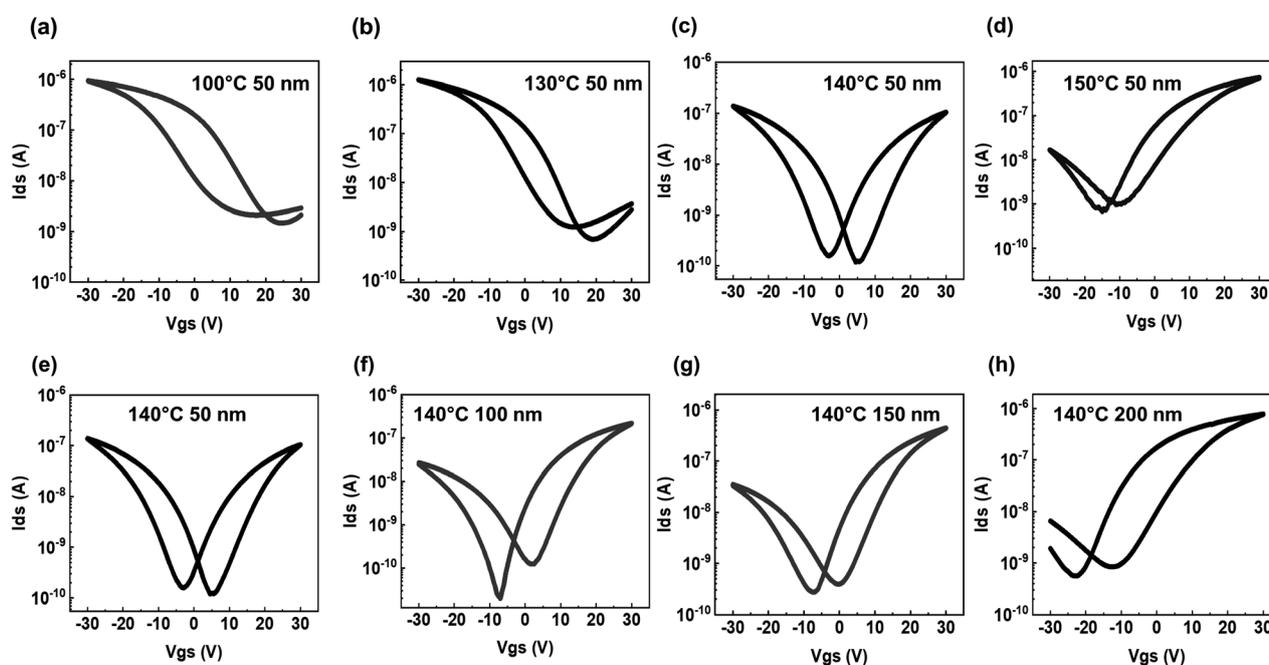
Fig. 2 (a)–(d) Transfer characteristics after 50 nm thickness Al<sub>2</sub>O<sub>3</sub> deposition at coating temperatures of 100 °C, 130 °C, 140 °C and 150 °C, respectively. (e)–(h) Transfer characteristics after the Al<sub>2</sub>O<sub>3</sub> deposition at 140 °C with coating thicknesses of 50 nm, 100 nm, 150 nm and 200 nm, respectively.
