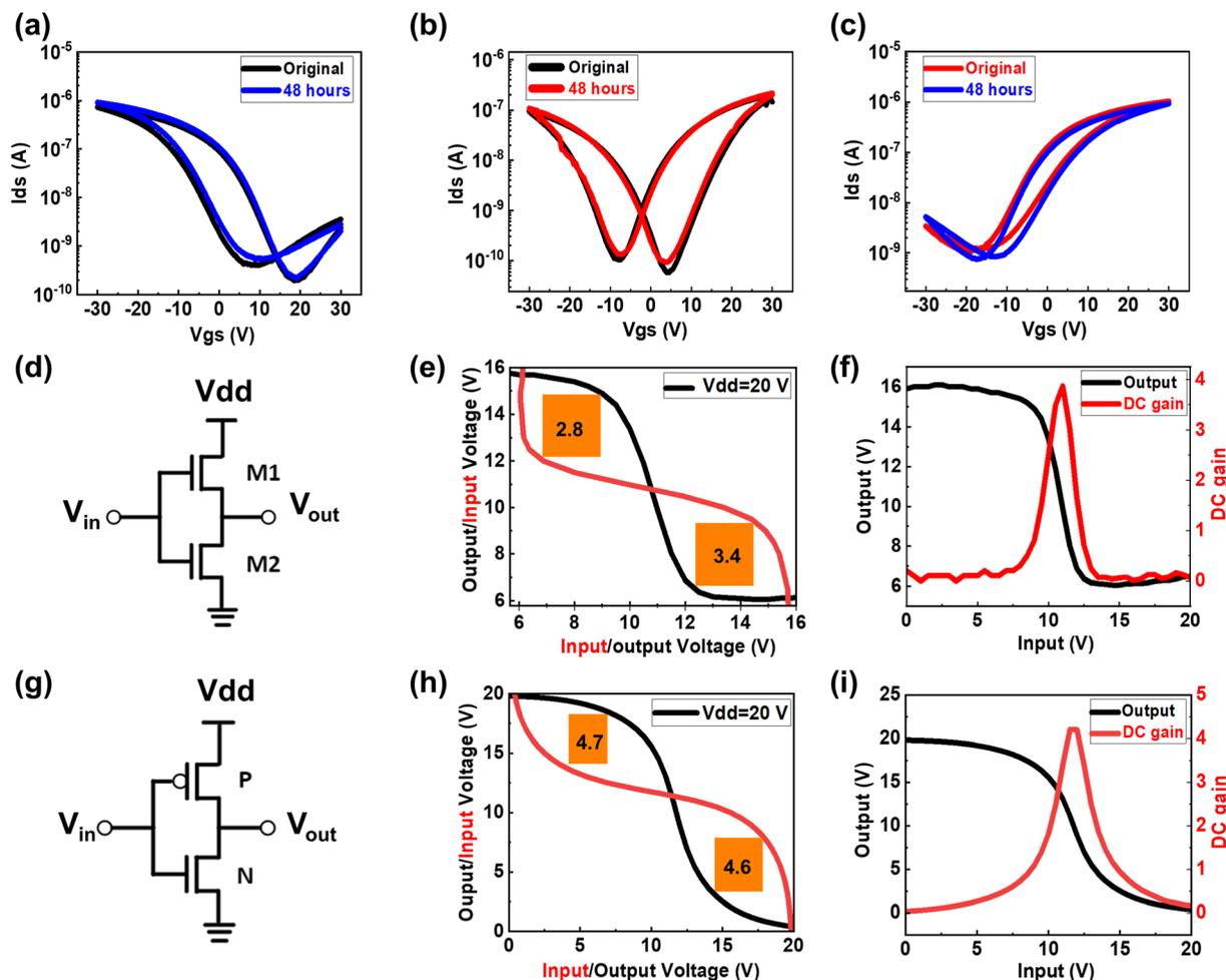
Fig. 4 (a) Stability test of  $\text{Al}_2\text{O}_3$  coated (a) p-type device, (b) ambipolar device, (c) n-type device. (d) Inverter circuit using two ambipolar devices. (e) Inverter VTC and noise margin at  $V_{\text{dd}} = -20$  V and (f) DC gain of the inverter from ambipolar TFTs. (g) Inverter circuit using CMOS device. (h) Inverter VTC and noise margin at  $V_{\text{dd}} = -20$  V and (i) DC gain of the inverter from the CMOS device.
