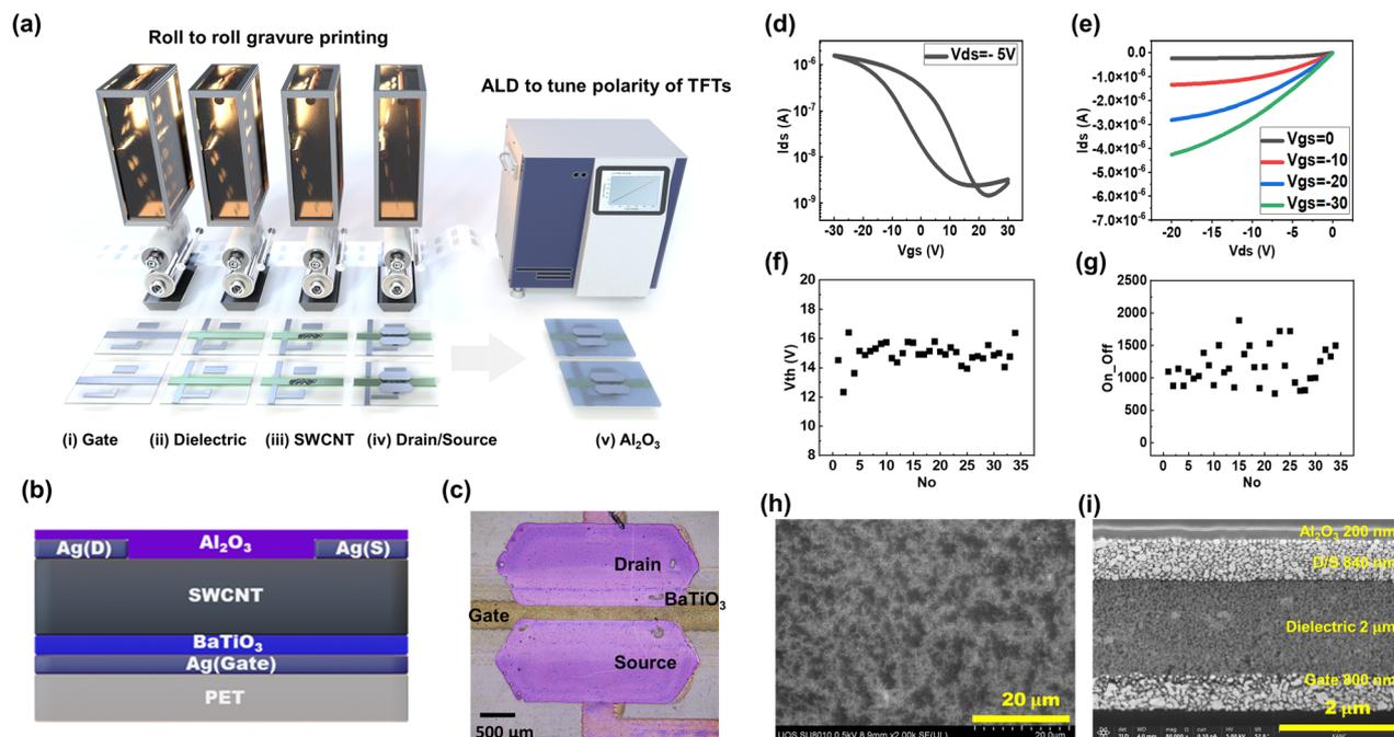
**Fig. 1** (a) Schematic of the fabrication process for SWCNT-TFTs through R2R printing and ALD process, (b) schematic cross-section view of an R2R printed SWCNT-TFT, (c) optical image of an R2R printed SWCNT-TFT, (d) typical transfer ( $V_{ds} = -5$  V) curve and (e) output curve of R2R printed SWCNT-TFTs, (f) scatter plots of  $V_{th}$ , (g) on-off ratio of 35 devices, (h) SEM image of SWCNT random networks, (i) FIB-SEM cross-sectional image of an R2R printed SWCNT-TFT.
