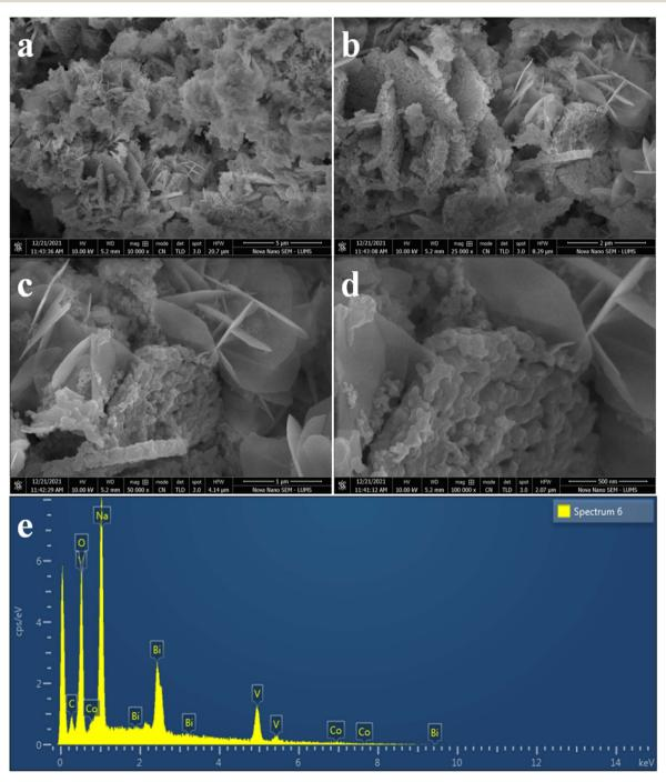
Fig. 3 SEM images of Co@Na-BiVO<sub>4</sub> microstructures (a) 5 μm (b) 2 μm (c) 1 μm and (d) 500 nm, whereas (e) represents the EDX analysis.
