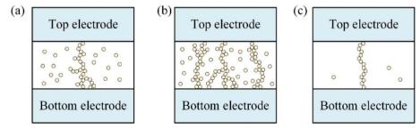
Fig. 3 The wire filament mechanism. (a) Initial resistance state (IRS). (b) Low resistance state (LRS). (c) High resistance state (HRS).
