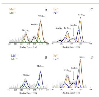
Fig. 6 High-resolution XPS spectra of Mn 2p in Mn<sub>0.2</sub><sup>2+</sup>Fe<sub>2.8</sub><sup>3+</sup>O<sub>4</sub> (A); Mn 2p in  ${\rm Mn_x}^{3+}{\rm Fe_{3-x}}^{3+}{\rm O_4}$  NPs (B); Fe 2p in  ${\rm Mn_{0.2}}^{2+}{\rm Fe_{2.8}}^{3+}{\rm O_4}$  (C) and Fe 2p in  ${\rm Mn_x}^{3+}{\rm Fe_{3-x}}^{3+}{\rm O_4}$  NPs (D).
