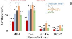
Fig. 7 In the presence of the tested agents (A) viability of tested Shewanella under sublethal dose of  $Cr^{6+}$  (B) removal of  $Cr^{6+}$  by Shewanella strains. \*P < 0.05 and \*\*P < 0.01 in relation to the impact of  $Mn_{0.2}^{2+}Fe_{2.8}^{3+}O_4$  NPs in each data set separately.
