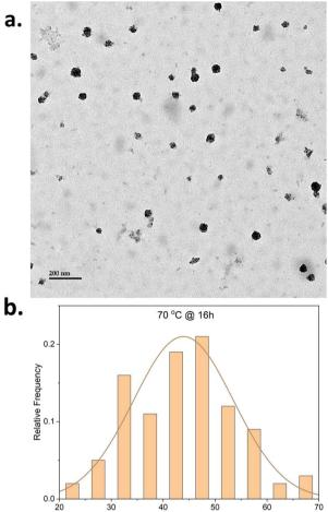
Fig. 1 (a) TEM image and (b) size histogram of CNPs synthesized at 70 °C for 16 hours.
