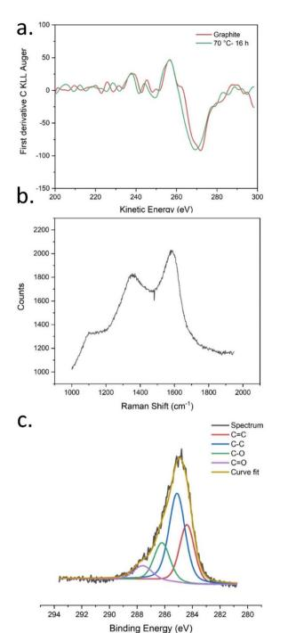
Fig. 2 (a) First derivative CKLL XAES spectrum for CNPs and graphite, (b) Raman spectrum, (c) high-resolution XPS C 1s spectra of CNPs synthesized at 70 °C for 16 hours.
