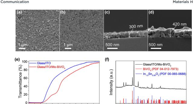
Fig. 3 FESEM images showing the morphology and thickness of the thin film. Top view image of (a) glass/ITO, (b) glass/ITO/Mo-BiVO<sub>4</sub>, and a cross section image of (c) glass/ITO, (d) glass/ITO/Mo-BiVO<sub>4</sub>. (e) UV-Vis spectra of glass/ITO compared to glass coated with ITO and Mo-BiVO<sub>4</sub>. (f) X-ray diffraction spectra of glass/ITO/Mo-BiVO<sub>4</sub>
