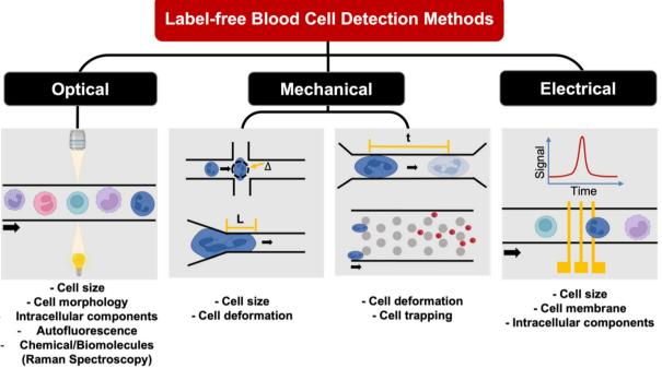
Fig. 8 Overview of microfluidic label-free single cell analysis.
