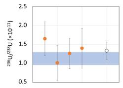
Fig. 6 Measurements of  $^{236}$ U/ $^{238}$ U isotope ratios in MTG sample. The open dot corresponds to the mean of the measurements (red dots). The blue rectangle highlights the certified value uncertainties. Uncertainties are extended with a coverage factor of 2.
