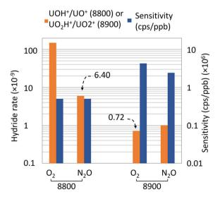
Fig. 2 Comparison of the hydride formation rate and sensitivity with Agilent 8800 ICP-MS/MS (left) from Jaegler *et al.* (2020) and Agilent 8900 ICP-MS/MS (right) using  $O_2$  or  $N_2O$  as a reaction gas in the CRC.
