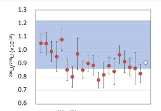
Fig. 5 Measurements of  $^{236}$ U/ $^{238}$ U isotope ratios in MBN sample. The open dot corresponds to the mean of the measurements (red dots). The blue rectangle highlights the certified value uncertainties. Uncertainties are extended with a coverage factor of 2.
