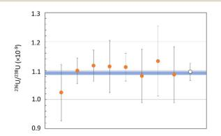
Fig. 3 Measurement of  $^{236}$ U/ $^{238}$ U isotope ratios in IRMM 075/6 certified reference material. The open dot corresponds to the mean of the measurements (red dots). The blue rectangle highlights the certified value uncertainties. Uncertainties are extended with a coverage factor of 2.
