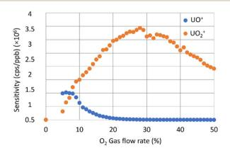
Fig. 1 Uranium oxide sensitivities using oxygen in the CRC, measured as UO+ (blue) or UO2+ (orange).
