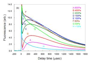
Fig. 3 (a) Temporal variation in the measured fluorescence signal of Ca and (b) its pressure dependence. Immediately after ablation, plasma emission was transmitted through the interference filter and overlapped with the fluorescence signal. The fluorescence signal had the highest intensity under about 100 Pa of helium.
