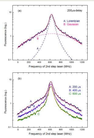
Fig. 8 (a) Fluorescence spectrum measured at 200  $\mu$ s delay. (A) Lorentzian and (B) Gaussian components obtained from least-square-fitting with eqn (3). (b). Fluorescence spectra measured at three different delay times along with the fitted curves. As the delay time increases, the Gaussian component disappears, whereas the Lorentzian component remains visible.
