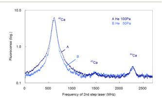
Fig. 12 Isotope-selective fluorescence spectra measured at a delay time of 1 ms under helium gas pressures of 100 and 50 Pa.
