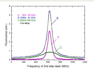
Fig. 9 Fluorescence spectra measured using various pressures and the curves fitted with the Voigt function. The intensities and linewidths vary with gas pressure, with the highest peak intensity occurring at about 100 Pa.
