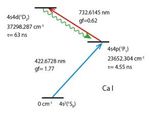
Fig. 2 Two-color two-step resonance excitation and fluorescence observation scheme of atomic Ca. Lifetimes ( $\tau$ ) of  $^1P_1$  and  $^1D_2$  levels were cited from ref. 43,44, oscillator strengths (gf) of the first and second transitions from ref. 45,46, level-energies, and transition wavelengths (in air) and configurations from ref. 47,48.
