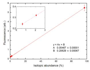
Fig. 13 Calibration curve between the fluorescence intensity and natural isotopic abundance of Ca. The inset is a magnified view of the <sup>42</sup>Ca and <sup>44</sup>Ca signals. The straight line is due to the least-square-fitting of these points, and a good correlation coefficient was obtained.
