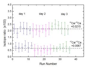
Fig. 15 Evaluation of reproducibility for three independent days. The  $^{44}$ Ca/ $^{40}$ Ca and  $^{42}$ Ca/ $^{40}$ Ca intensity ratios are in good agreement with the natural isotope ratios, and the measurement accuracy is about 10%.
