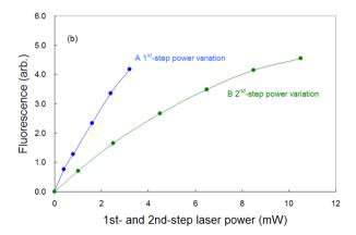
Fig. 4 Dependence of the fluorescence intensity with the pulse energy of YAG laser (a) and powers of diode lasers (b). In (a), the fluorescence signal starts to appear at about 0.1 mJ and is saturated at 0.3 mJ or more. In contrast, in (b), the fluorescence intensity increases consistently as the first-step and second-step laser powers increase. In (b), the power of the remaining diode laser was fixed at its maximum value (3 mW and 10.5 mW) during this measurement.
