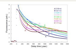
Fig. 5 Temporal variation in the fluorescence signal measured with various ablation pulse energies. The fluorescence intensity around 500  $\mu s$  starts to decrease with increasing ablation energy when the energy exceeds 0.3 mJ, while the intensity around 1800  $\mu s$  increases consistently.
