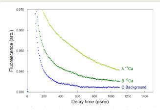
Fig. 14 Typical temporal profiles of the <sup>42</sup>Ca and <sup>44</sup>Ca fluorescence signals and a background signal. We evaluated the signal-to-noise ratio of the <sup>44</sup>Ca signal and the limit of detection from these curves.
