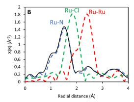
Fig. 3 XANES (A) and EXAFS (B) data for CBV-100-Ru(bipy)<sub>3</sub> (solid black) in comparison with reference samples (dashed lines): Ru(bipy)<sub>3</sub><sup>2+</sup>@EMC-1,<sup>27</sup> blue; RuCl<sub>3</sub>, green; Ru-foil, red.
