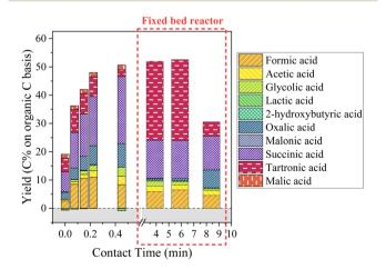
Fig. 13 Aliphatic compounds production during KBL catalytic oxidation. Operating conditions: 150 °C, 20-80 bar air, dry matter concentration 5 g L<sup>-1</sup>, catalyst CuO/TiO<sub>2</sub>.
