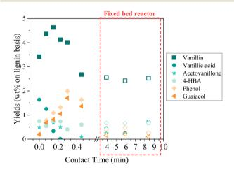
Fig. 12 Details of phenolics production during KBL catalytic oxidation. Operating conditions: 150 °C, 20-80 bar air, dry matter concentration 5 g L<sup>-1</sup>, catalyst CuO/TiO<sub>2</sub>.
