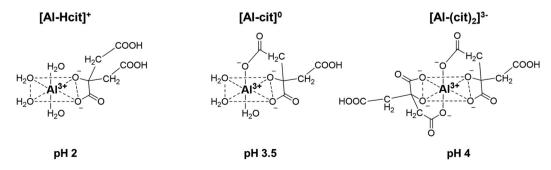
Fig. 2 Structures of different Al-citrate complexes and pH values at which their presence is most dominant. 50,51
