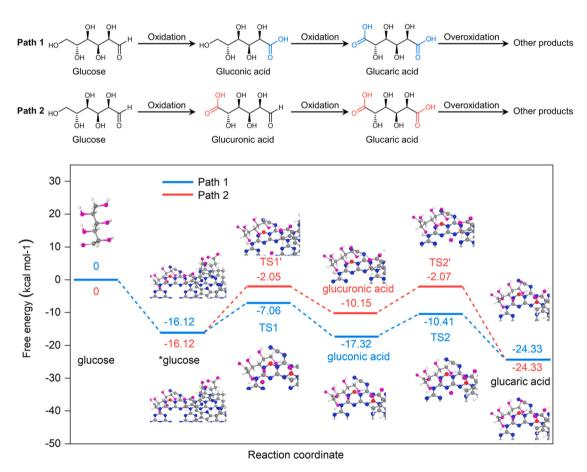
Fig. 10 At the top of the figure, glucose oxidation pathways over Ce6@BNCN proposed by Bai et al. are depicted. At the bottom, quantum chemical calculations for the proposed pathways are shown. Reproduced with permission from ref. 102. Copyright 2021, Elsevier.
