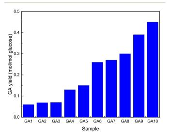
Fig. 3 Increase in GA yield by metabolic engineering of E. coli. The graph was drawn from data reported by Su et al. 52 GA1-unaltered enzyme, GA2-T7 promotor included in the plasmid, GA3-laclq removed, GA4-uxaC additionally removed, GA5-gudD additionally removed, GA6-8-(zwf and pgi) additionally removed, GA9-ribosome binding sites optimized, and GA10-inclusion of the nox gene and improved agitation.
