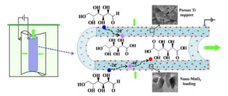
Fig. 12 Schematic representation of the nano-MnO<sub>2</sub>-loading tubular porous titanium electrode used by Bin et al. Reproduced with permission from ref. 113. Copyright 2014 Elsevier.
