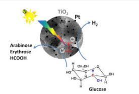
Fig. 8 Graphical illustration of the photoconversion of Glc in the presence of Pt-loaded  $TiO_2$  catalysts. Reproduced with permission from ref. 94. Copyright 2016, Elsevier.
