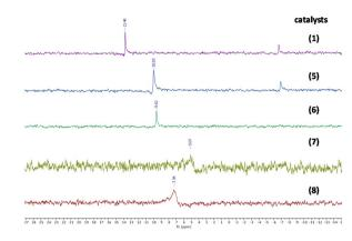
Fig. 4  $^{95}$ Mo-NMR spectra of [MoO<sub>4</sub>]<sup>-</sup> ILs (see the ESI for the complete spectra, Fig. S9, S30, S25, S34 and S38†).
