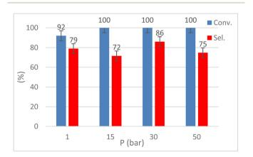
Fig. 8 Pressure screening for CO<sub>2</sub> insertion into 1,2-epoxyhexane (EH) to obtain hexane carbonate (HC). Reaction conditions: EH (4 mmol), 1 (2.5 mol%), T = 120 °C, t = 9 h, p = 1-50 bar (CO<sub>2</sub>), solventless conditions. Conversion and selectivity were calculated by <sup>1</sup>H-NMR.
