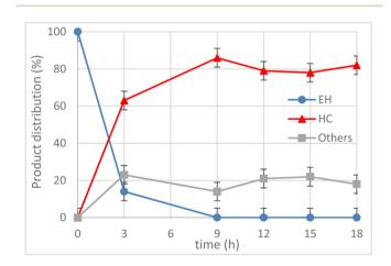
Fig. 7 Effect of the reaction time on  $CO_2$  insertion into 1,2-epoxyhexane (EH) to obtain hexane carbonate (HC). Reaction conditions: EH (4 mmol), 1 (2.5 mol%),  $CO_2$  (30 bar), T = 120 °C, t = 3-18 h, solventless conditions. <sup>a</sup> Determined by GC-FID.
