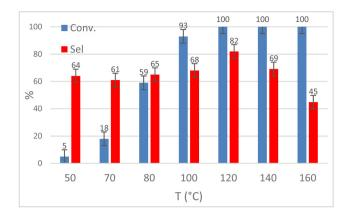
Fig. 6 Effect of the temperature on  $CO_2$  insertion into 1,2-epoxyhexane (EH) to obtain hexane carbonate (HC). Reaction conditions: EH (4 mmol), 1 (2.5 mol%),  $CO_2$  (30 bar), t = 18 h, T = 50-160 °C, solventless reaction. Conversion, selectivity and yield were calculated by  $^1H$ -NMR.
