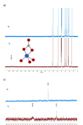
Fig. 9  $^{13}$ C-NMR (a) and  $^{95}$ Mo-NMR (b) analyses of [N<sub>8881</sub>]<sub>2</sub>[MoO<sub>4</sub>] before (blue) and after (red) treatment with CO2. Operative conditions:  $[N_{8881}]_2[MoO_4]$  0.4 M in DMSO-d<sup>6</sup>, T = 25 °C,  $p^0(CO_2) = 5$  bar.
