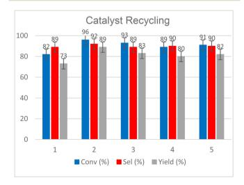
Fig. 11 Catalyst recycling tests for CO<sub>2</sub> insertion into 1,2-epoxyhexane (EH) to obtain hexane carbonate (HC). Reaction conditions: EH (20 mmol), 1 (2.5 mol%), T = 120 °C, t = 9 h,  $p^{0}(CO_{2}) = 30$  bar, solventless conditions. Conversion, selectivity and yield were calculated by <sup>1</sup>H-NMR.
