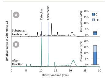
Fig. 7 HPLC-UV analysis and quantification of catechin (C) and epicatechin (EC) of two solutions: (A) crude larch bark extract, as obtained via Soxhlet extraction with methanol, and (B) the product mixture after depolymerisation-hydrogenation of a crude larch bark extract. Reaction conditions: 60 mL crude larch bark extract in methanol (4.8 g extractives per L), 30 bar H<sub>2</sub>, 25 mg Pd/C, 200 min reaction time.
