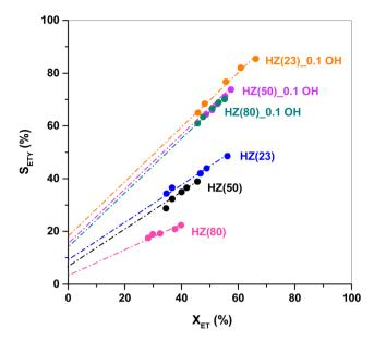
Fig. 7 ETY selectivity ( $S_{ETY}$ ) as a function of ET conversion ( $X_{ET}$ , changed with WHSV) over HZ(23), HZ(50), HZ(80), HZ(23)\_0.1 OH, HZ (50)\_0.1 OH and HZ(80)\_0.1 OH. Test conditions: 225 °C, total pressure  $\sim$ 1 bar. WHSV = 17.9-89.1 h<sup>-1</sup>.
