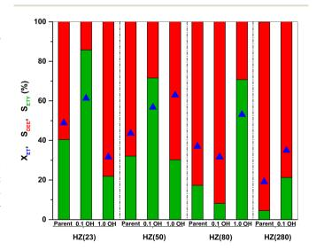
Fig. 1 Conversion of ET (blue), selectivity of ETY (green) and of DEE (red) provided by parent HZSM-5 catalysts and by their counterparts treated in alkaline solution (values estimated at steady-state of reaction (5-6 h)). Test conditions: 225 °C, 1 bar, WHSV = 35.7 h<sup>-1</sup>.
