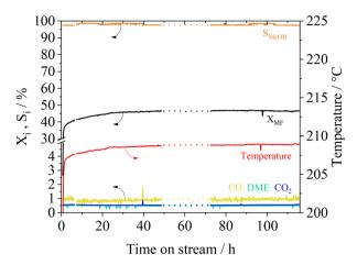
Fig. 8 Conversion and selectivity over time with the Cu<sub>0.9</sub>Al<sub>2</sub>O<sub>4</sub> catalyst, reaction conditions: T = 208 °C, p = 10 bar<sub>q</sub>,  $V_{\text{total}} = 704$  ml<sub>N</sub> min<sup>-1</sup>,  $n_{\rm H_o}$ :  $n_{\rm MF}$  = 5.8,  $m_{\rm cat.}$  = 0.5 g; dotted line: interpolation of experimental data during a temporal breakdown of our reaction analytics.
