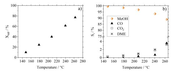
Fig. 6 Temperature influence on (a) conversion and (b) selectivity in pure MF hydrogenolysis using  $Cu_{0.9}Al_2O_4$ ; reaction conditions: T = 150-260 °C, p = 10 bar<sub>g</sub>,  $V_{\text{total}} = 704$  ml<sub>N</sub> min<sup>-1</sup>,  $n_{\text{H}_2}$ :  $n_{\text{MF}} = 5.8$ ,  $m_{\text{cat.}} = 0.5$  g.
