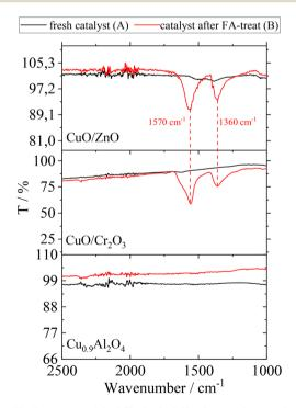
Fig. 4 ATR-IR spectra of CuO/ZnO, CuO/Cr<sub>2</sub>O<sub>3</sub> and Cu<sub>0.9</sub>Al<sub>2</sub>O<sub>4</sub> before (A) and after (B) contact with FA; assignment of peaks: carboxylate ion of formate species (1570 cm<sup>-1</sup> asymmetric stretch and 1360 cm<sup>-1</sup> symmetric stretch).33
