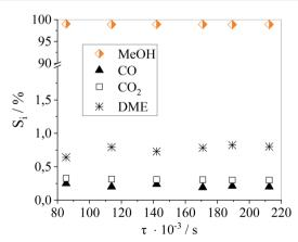
Fig. 7 Effect of residence time variation on (a) conversion and (b) selectivity in pure MF hydrogenolysis using Cu<sub>0.9</sub>Al<sub>2</sub>O<sub>4</sub>; reaction conditions: p = 10 bar<sub>g</sub>, T = 188 °C,  $n_{H_2}$ :  $n_{MF}^{-1} = 5.6$ ,  $V_{total} = 566-1408$  ml<sub>N</sub> min<sup>-1</sup>,  $m_{cat.} = 0.32$  g.
