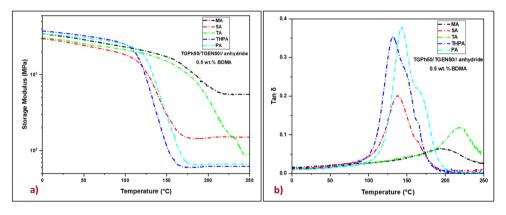
Fig. 3 Storage moduli (a) and  $\tan \delta$  (b) curves of the TGPh50/TGEN50//anhydride thermosets.
