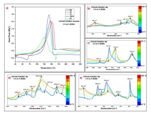
Fig. 2 (a) Dynamic DSC thermograms obtained during the crosslinking of TGPh50/TGEN50//anhydride formulations initiated by 0.5 wt% BDMA, and the temperature-dependent FT-IR spectra of the TGPh50/TGEN50//MA system during curing in the regions (b) 3800-2800 cm<sup>-1</sup>, (c)  $1950-1550 \text{ cm}^{-1}$ , (d)  $1350-1000 \text{ cm}^{-1}$ , and (e)  $1000-650 \text{ cm}^{-1}$ .
