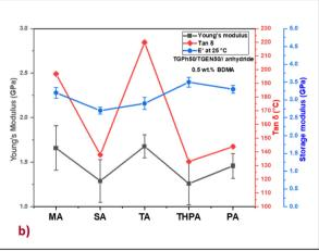
Fig. 4 (a) Representative stress-strain curves and (b) Young's modulus,  $\tan \delta$  and storage modulus (E') at 25 °C for the designed thermosets.
