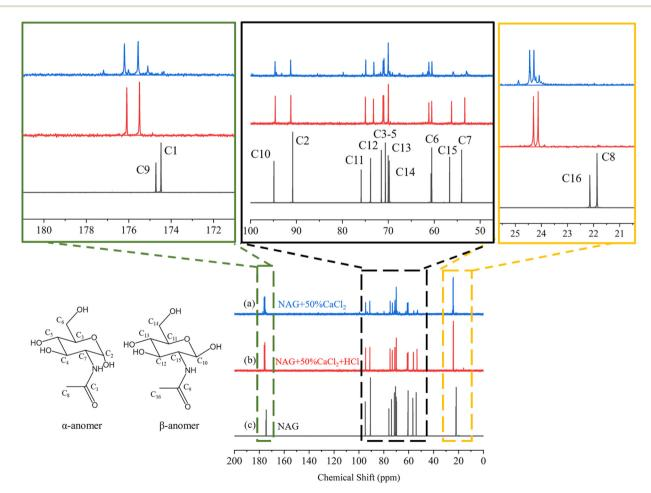
Fig. 4 13C NMR of (a) NAG, (b) NAG with HCl (30 mM HCl) and 50% CaCl<sub>2</sub> and (c) NAG with 50% CaCl<sub>2</sub>. The solutions were prepared using D<sub>2</sub>O.
