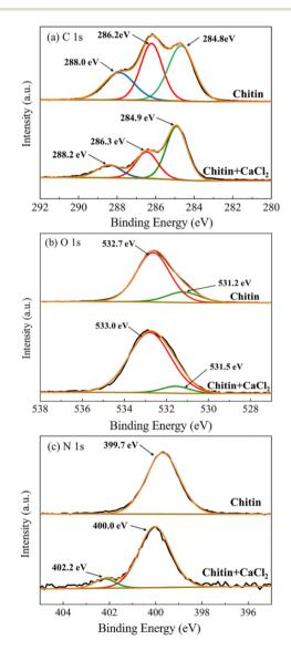
Fig. 5 (a) C 1s, (b) O 1s, and (c) N 1s XPS patterns of chitin and chitin— $CaCl_2$ .
