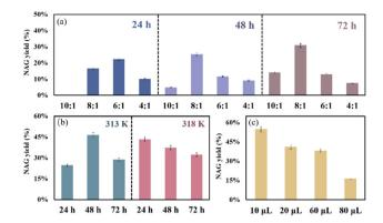
Fig. 2 The NAG yield under different chitin aging conditions. (a) At RT, the C/A ratio was 10:1, 8:1, 6:1 and 4:1 and the aging time was at a range from 24 h to 72 h; (b) at 313 K and 318 K, the C/A ratio was 8:1 and the aging time was at a range from 24 h to 72 h; and (c) at 313 K, the C/A ratio was 8:1, and the aging time was 48 h and the volume of water addition was 10 uL, 20 uL, 60 uL and 80 uL. Other reaction conditions: 0.2 g of chitin was added into 4 mL of solvent and heated at 393 K for
