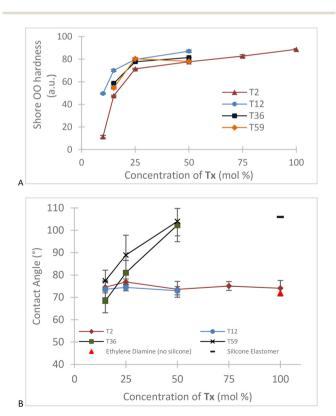
Fig. 2 Changes in (A): hardness and (B): contact angle with different ratios of 2 to a series of aminosilicones.
