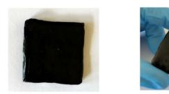
Fig. 4 Lignin shaping on hot plates after hydroesterification of methyl 10-undecenoate - upscaling of the experiment from Table 4 entry 4.
