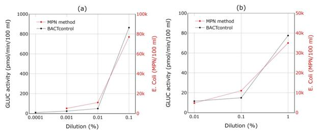
Fig. 7 The relationship between the GLUC activity and *E. coli* with the MPN method for different dilution levels of fresh sewage with surface water: a) 0.001–0.1%, b) 0.01–1%.
