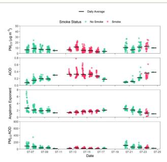
Fig. 6 Time-series plots of PM<sub>2.5</sub>, AOD, Angstrom exponent, and PM<sub>2.5</sub>: AOD ratio from July 6, 2021, to July 24, 2021, from four CEAMS sites in Southern California, colored by HMS-derived smoke status. Measurements are from four AMODv2s (Fig. 1). Note that measurements on July 12, 2021, were from a single AMODv2 started early by the CEAMS participant.
