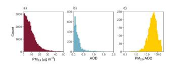
Fig. 3 Histograms of (a) PM<sub>2.5</sub>, (b) AOD at 500 nm, and (c) PM<sub>2.5</sub>: AOD ratio for all valid measurements across all CEAMS sites for June-August 2021 deployment. Counts represent measurements collected at 20 minute intervals.
