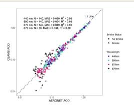
Fig. 4 Scatter plot of CEAMS and AERONET AOD measurement pairs occurring within 180 seconds and 25 km of each other. N= number of paired triplicate measurement points; MAE = mean absolute error in dimensionless AOD units. Table with correlations for smoke and no smoke days is provided in Table S1.†
