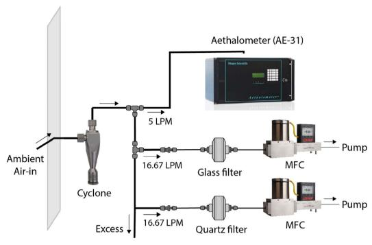
Fig. 1 Sampling set-up used for collecting ambient particulates on glass and quartz-fiber filters. An aethalometer (AE-31) parallelly measured BC for training filter R to BC model and to validate image-based BC. A cyclone was used at the collective inlet to allow only PM<sub>2.5</sub> during sampling.
